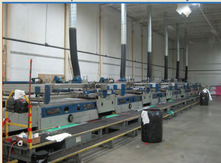
Six-color screen press with 85-inch, UV-arc system
