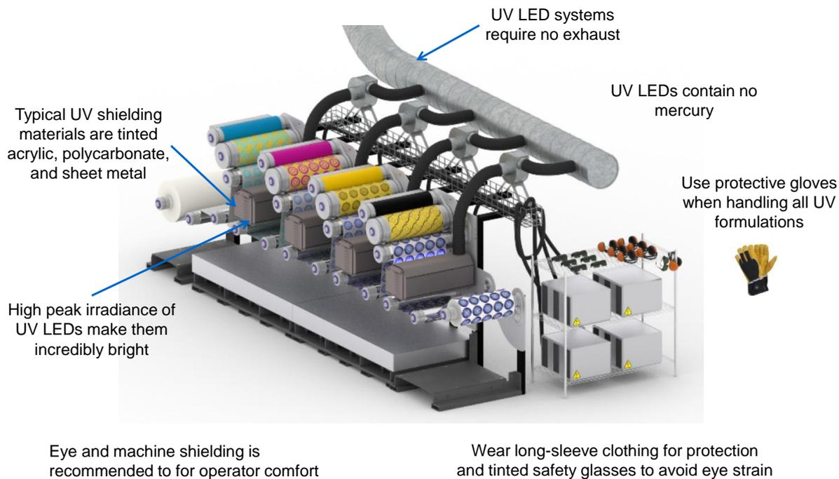
**Figure 5: UV LED Systems are Safer Installations and Result in Safer Operation.**
